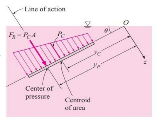
vertical location of the line of action is determined by equating the moment of the resultant force to the moment of the distributed pressure force about the x-axis.
